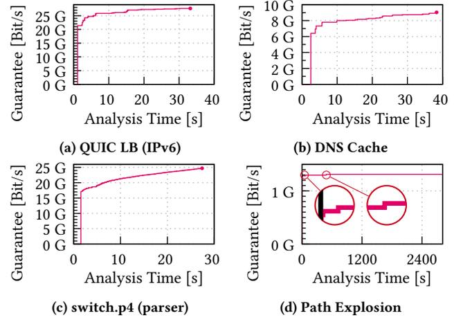
**Figure 7: The throughput guarantee improves until a satisfiable path is found (a-c) or the the analysis is aborted (d).**
