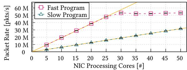
Figure 4: The throughput capacity when using different numbers of NIC cores is limited by the maximum packet rate of the NIC of 54.4M pkts/s. Below that, packet rates are proportional (orange lines) to the number of cores. fast program: 1.92M pkts/s/core with  $R^2 = 0.999949$  slow program: 0.63M pkts/s/core with  $R^2 = 0.999985$
