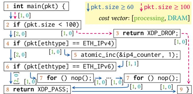
**Figure 6: The resulting CFG of the program from Figure 2. A realistic example would use NFP bytecode.**
