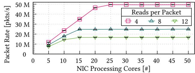
**Figure 5: The DRAM bottleneck is observable when enough processing cores are used. The memory engine then performs at a rate of 197.4M ops/s to 199.7M ops/s independent of the number of reads per packet.**
